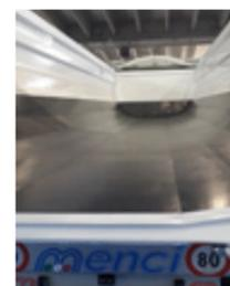
The completely smooth **HMPE** surface allows for **high fluidity**.
